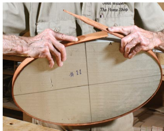
Wrap it up. The 1" foam core is used as a bending form. The start mark is found by marking the length of the finger pattern for each size tray on the foam core as you can see. When the wrap is done, the main tack line will fall on the centerline.
