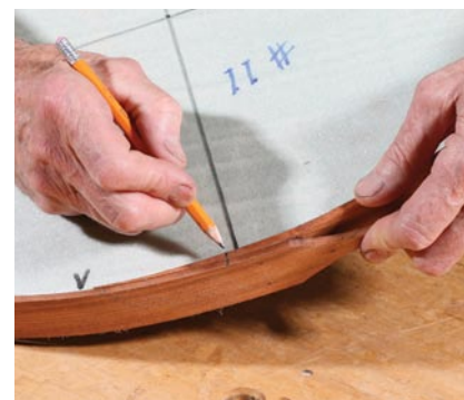
Mark it. Record your tight wrap by a pencil mark. Remove the band from the foam core, and use this mark as a reference for sizing the tray. By going \frac{1}{8} " past the mark when tacking, the resulting size will fit snugly back on the form.
