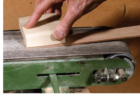
Feathered. The inside square end is feathered to give a smooth inside curve to the tray. Here the sanding tapers back 2\frac{1}{2} " to 3 " and removes thickness to almost nothing at the end.
