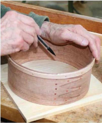
**Mark a circle.** Once the band and rim are thoroughly dry, the box will hold its round shape. So you can use it as the template for marking the bottom board.
