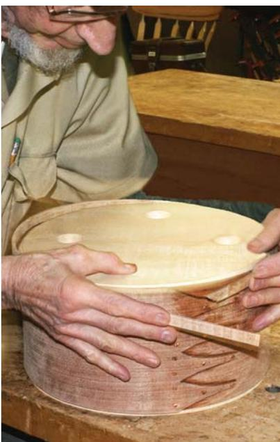
**Add the rim.** The rim gets tucked into the curve of the top finger and ends with a 4" lap that will project about 1" beyond the fingers. After bending the rim in place, remove the top shaper and hold the rim in place (a spring clamp might help) as you drill 1/16"-diameter pilot holes every 3" for the escutcheon pins (with three holes 2" apart at the lap).
