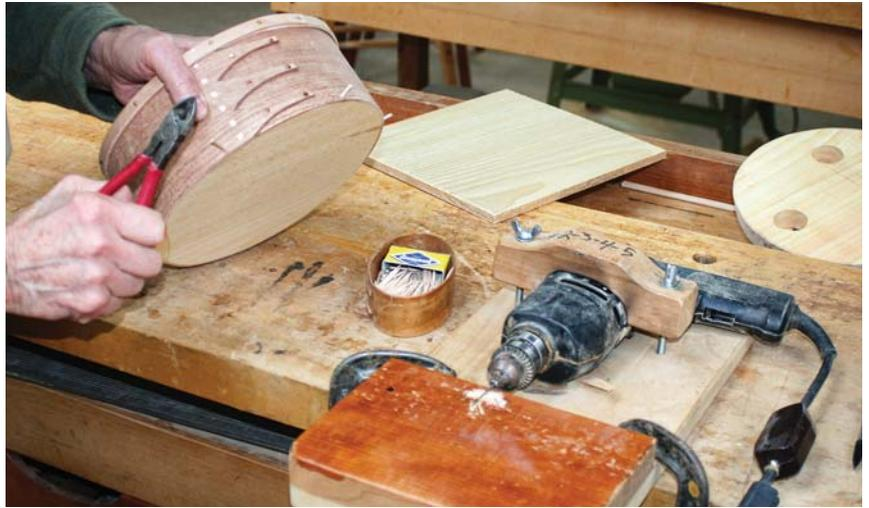
**Secure the bottom.** I use toothpicks to secure the bottom, drilling  $\frac{5}{64}$ " pilot holes every 2"-3" around the box, centered in the thickness of the bottom. After tapping the toothpicks in place, I use side cutters to snip them off, then sand smooth.
