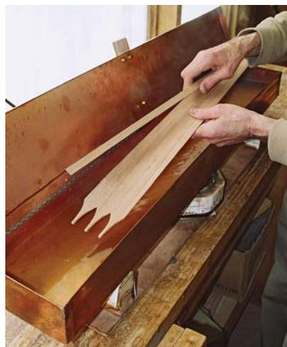
**In hot water.** My copper water tray sits on a hot plate, with wood blocks under each end for stability. A full boil is not necessary; 180° F will soften the lignin sufficiently for bending in about 10-20 minutes.
